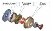
The high capacity torque converter with optimized turbine set grille structure improves the double-pump confluence system to maximize the transmission efficiency and minimize the energy consumption. In addition, the reduced thermal balance temperature of the hydraulic oil effectively improves the reliability of the related parts.
